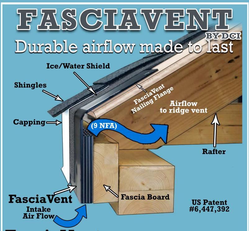
Fascia Vent allows air to enter through the fascia board, under the roof decking structure and out the ridge vent or other installed exhaust device. Your gutter can be installed directly onto Fascia Vent or a metal capping can cover the vent.
