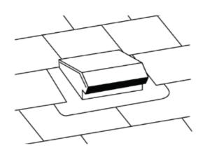
8. Apply nails to secure the SnapCap to the roof. Use caulk or roof cement to seal nail heads and shingles to the top and sides of the vent.
