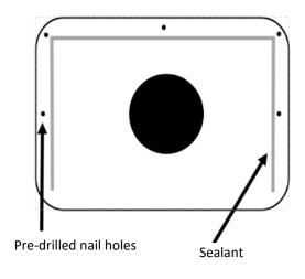
7. Align the vent over the opening. Place the upper flange underneath the shingles and the lower flange over the shingles. Trim shingles around the vent as needed.
