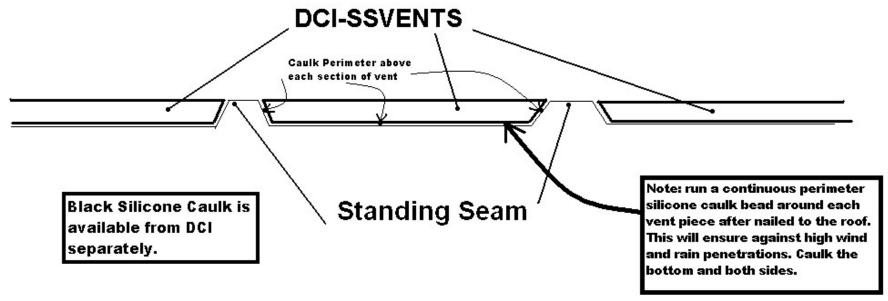
Note: Install capping metal over DCI-SSVENTS that complement the standing seam roof metal. For added ventilation, install SmartRidge II over the DCI-SSVent with external edges of the SmartRidge flush or extending beyond the lower DCI-SSVent.
