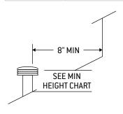
Note: Vents larger than 12" must exhuast a minimum of 12" higher than any part of the roof within 10'
