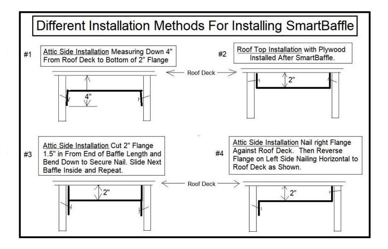
Use 1/2" staples or 1" screws or 1.25" roofing nails to attach Baffles to side wood rafters. Cuts can easily be made with a retractable type utility knife. Bends can be made by cutting halfway through plastic on the side opposite the bend direction of choice.
