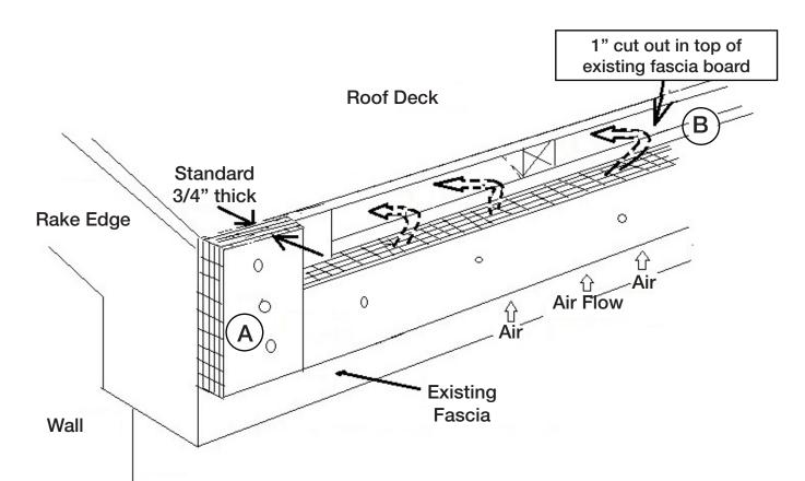
Prior to installing Fascia Strip Vent, Cut 1" off the top of the fascia board, stopping 12" in from the edges and corners. Cut a strip to use as an end cap from the roof edge to the bottom of the vent as shown (A). All rake edges require this end cap. The Fascia Strip Vent does not extend further than the bottom of the 1" cutout as shown (B). Nail vents every 6" as shown. Nail end caps with 2 or 3 nails. Cover entire face with a new full size fascia board or aluminum capping extending onto roof.
